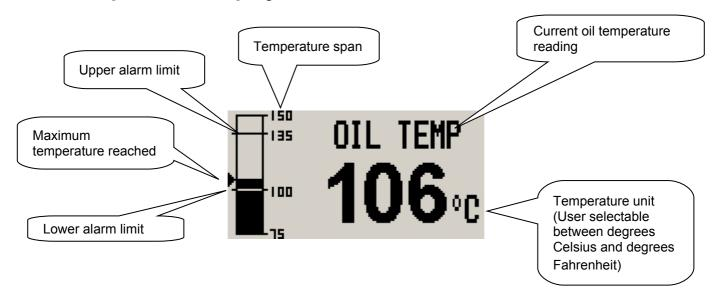
The EMS-1 uses standard automotive oil temperature senders to display the oil temperature. All oil temperature parameters can be changed in the "OIL TEMP SETUP" menu. The EMS-1 also contains fail safe oil temperature inputs to alert the user when the sender has been disconnected or faulty. The EMS-1 oil temperature VDO reading is linearized for a VDO part number VDO 323/801/009/001C oil temperature sender. A custom user sender can also be used.
