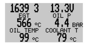
This screen displays all the measured parameters simultaneously.
