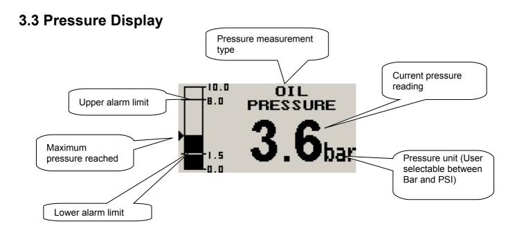
The EMS-1 uses standard automotive pressure senders to display the pressure. The EMS-1 supports 2, 5 and 10 Bar VDO senders or a custom user definable pressure sender curve.
