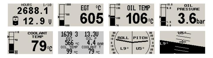
The information display screens can be viewed by pressing the up and down buttons in the normal run mode. The EMS-1 can also be set up to scroll through the screens automatically (this can be setup under the "UNIT SETUP" menu).
