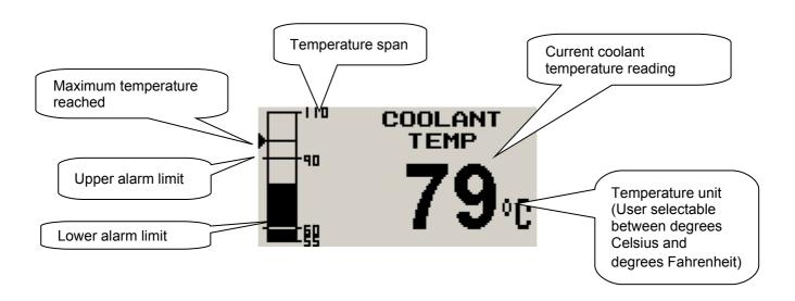
The EMS-1 uses standard automotive engine coolant temperature senders to display the coolant temperature. All coolant temperature parameters can be changed in the "COOLANT TEMP SETUP" menu. The EMS-1 also contains fail safe coolant temperature and coolant level inputs to alert the user when the sender has been disconnected or faulty. The EMS-1 caters for the VDO 120°C and the VDO 150°C temperature sender. A custom user sender can also be used.
