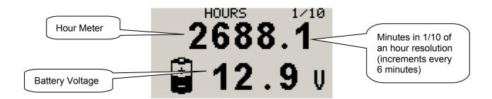
The EMS-1 can measure the vehicle's battery voltage in the range of 8V to 30Vdc and has built in over-voltage and reverse voltage protection. The EMS-1 contains a programmable low/high voltage alarm to automatically catch alternator failures, drive belt failures and bad batteries.
