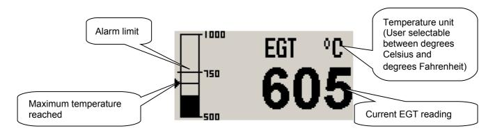
The EMS-1 can use K-Type or J-Type thermocouples to display the EGT temperature. The EMS-1 contains precision instrumentation electronic circuitry to amplify and linearize the thermocouple sensor. The EMS-1 also has built in cold junction compensation to make the EGT reading as accurate as possible. All EGT parameters can be changed in the "EGT SETUP" menu.
