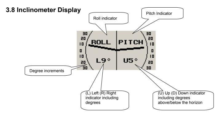
The left dial indicates the ROLL (left/right movement) of the vehicle, and the right side the pitch (up/down movement) of the vehicle. The horizon calibration in the menu system must be done at the time of installation to align the sensors to the horizon.
